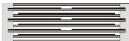
Extended metallized film design with internal series connection (series connection of elements)
