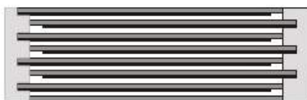
Extended metallized film design
